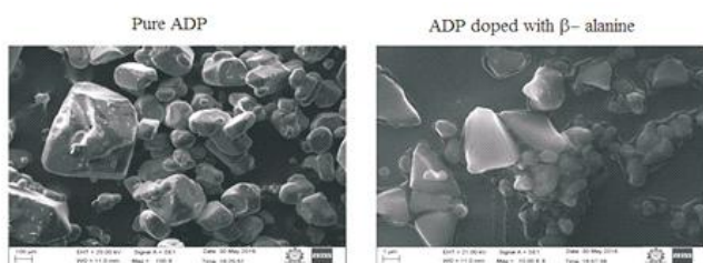
Fig. 9: SEM image of pure ADP and ADP doped with \beta -alanine crystal.
